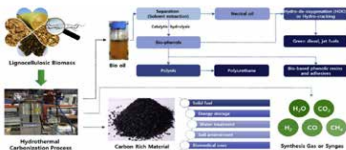
Khan et al. 2019. Bioenergy 130, 105384. Fig. 1. Graphic diagram of workable models about the carbon rich materials manufacture, applications
