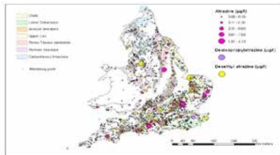
Figure 7.3 Distribution of mean concentrations of atrazine and its metabolites in the Environment Agency groundwater organic micropollutant database
