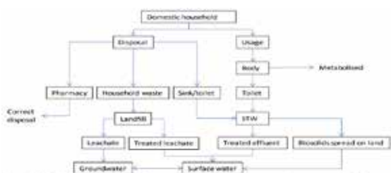
Figure 5.2 Pathways for domestic pharmaceuticals to reach the aqueous environment (adapted from Bland and Voshell, 2005)
