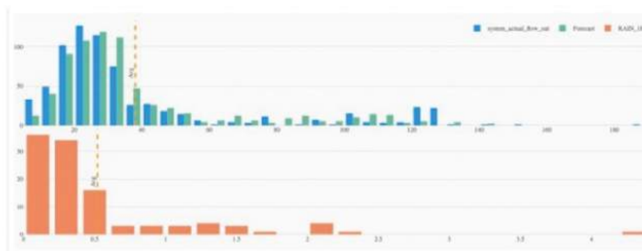
Figure 3 Distribution of observed sewer volume forecasts and rain values. The x-axis in top plot shows the observed actual flow and the corresponding forecast results. The x-axis in the bottom plot shows the amount of rain. The y-axis in two plots show the frequency of observing a specific value in x-axis.
